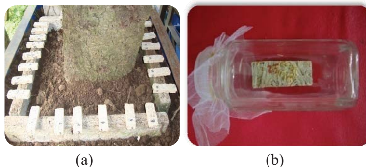
Figure 1. Set-up of accelerated test on the resistance of wood wool cement board (WWCB) to: (a) subterranean termites M. losbañosensis and (b) drywood termites C. dudleyi .
